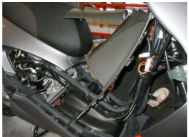
**7.1.6. REMOVING THE FRONT INNER SHIELD**
