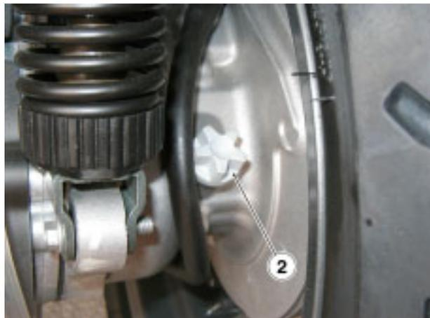
**IMPORTANT** To facilitate the filling of the oil pan, rotate the wheel with your hands.
