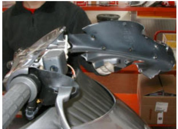
**7.1.14. REMOVING THE REAR HANDLEBAR COVER**
